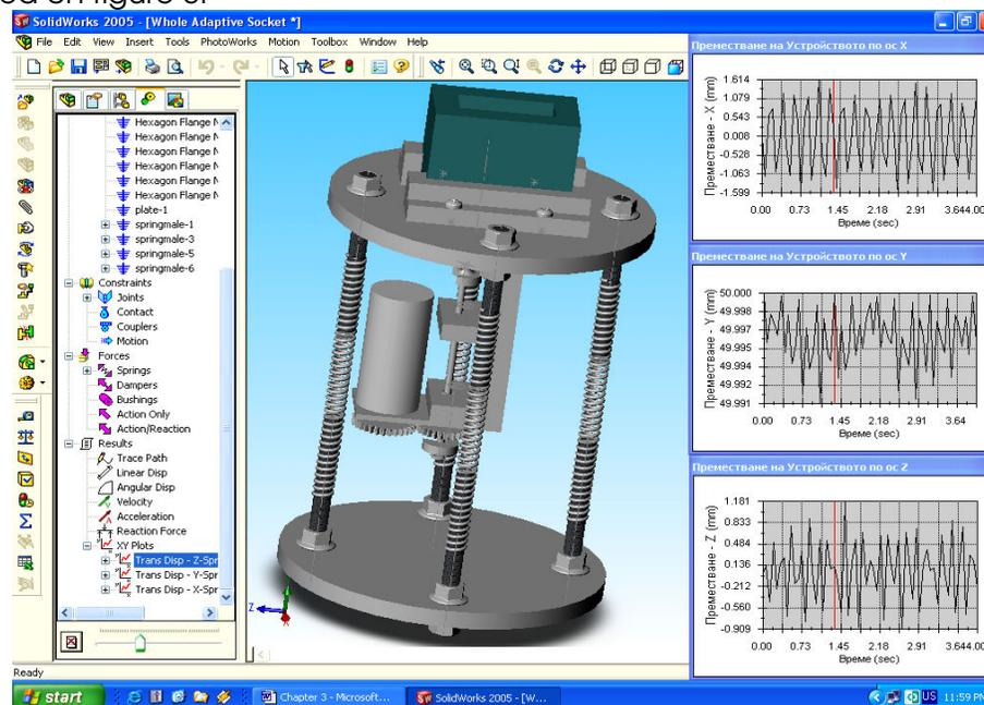
Figure 6. Dynamic model and simulation of the operation of adaptive socket
