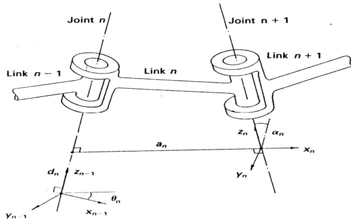
FIGURE 4. Denavit Hartenberg coordinate systems and parameters of the robotic system
