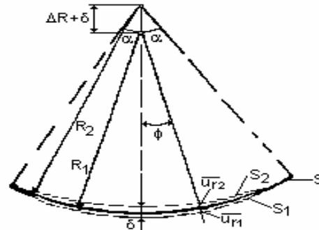
Fig.2. The deformed state in the contact zone
