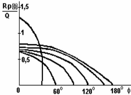
Fig.3. The Persson's contact pressure distribution
