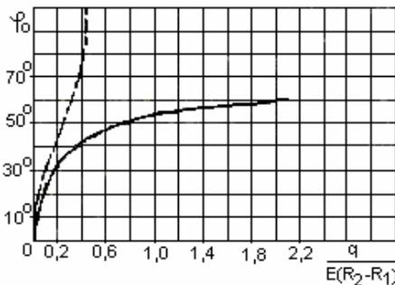
Fig.6. Comparison between Steuermann's and Hertz's results
