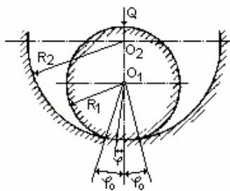
Fig.5. Contact between a cylinder and a cylinder cavity
