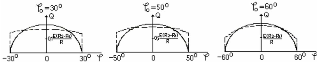
Fig.7. The distribution  $Q(\varphi)$  according to Pantou's (non-continuous line) and Steuermann's theories (continuous line)
