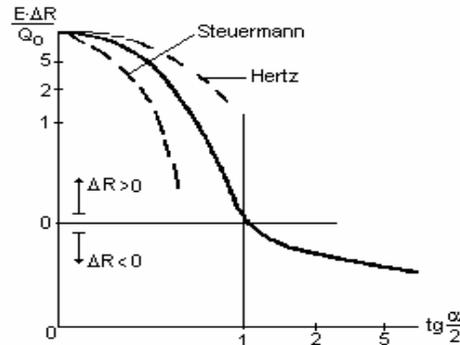
Fig.4. The variation of the contact angle limits (the arc)  $\alpha$  function of the normal surface loading  $Q$
