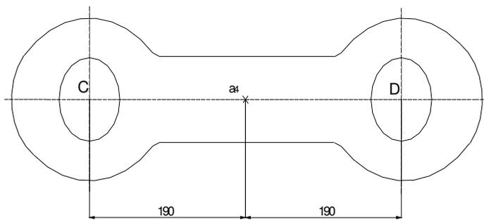
Figure 4. Gravity centre of the element (4) (long driving rod)
