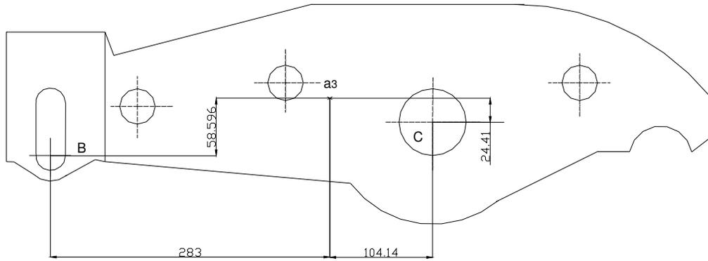
Figure 3. Gravity centre of the element (3) (upper arm)
