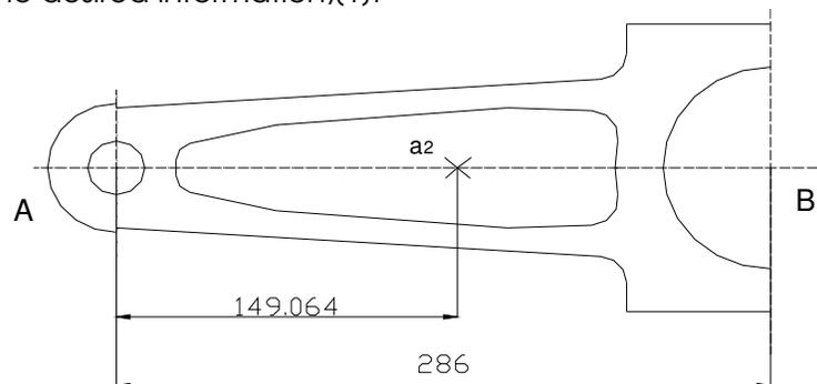
Figure 2. Gravity centre of the element (2) (short driving rod)
