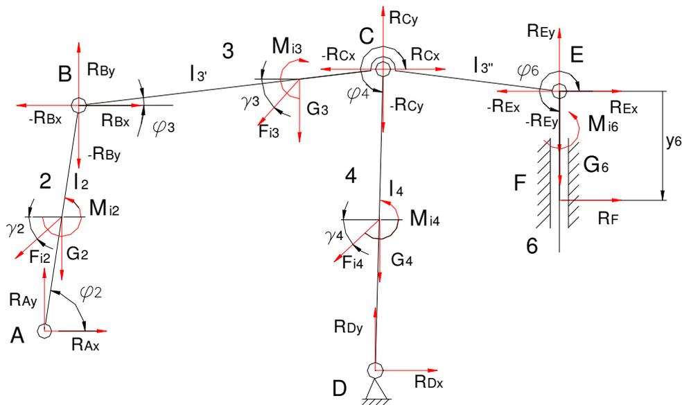
Figure 7. Loading Scheme of ABCDE triad
