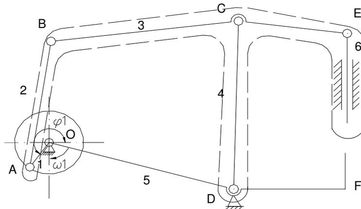
Figure 1. Kinetic Scheme of the laboratory model of the 8000kN shear
