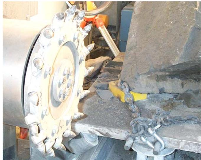
**FIGURE 1. TYPICAL EXAMPLE OF MECHANICAL INTERACTION WITHIN THE BITS AND HARD ROCK (I.E. ORE DISINTEGRATION PROCESS)**
