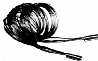
FIGURE 4. Fitting of the tensiometer for the working housing of the experimental rolling-mill
