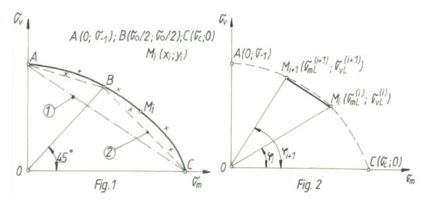
Therefore, the experimental determination of points on the Haigh type diagram and the approximation of this diagram through a polygonal line, will nonetheless contribute to the perfecting process entailed by the value of the safety coefficient.
