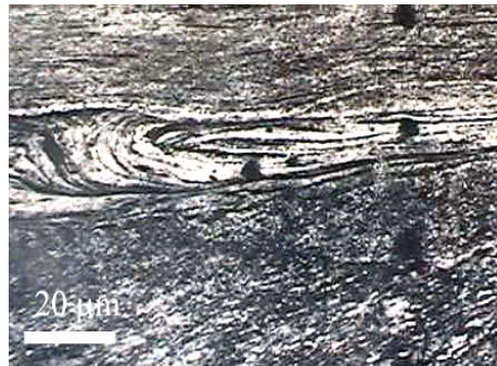
FIGURE 7. VORTICAL DEFORMATION MODE AT THE INTERFACE BETWEEN NANOCRYSTALLINE LAYER (TOP) AND PLASTICALLY DEFORMED ZONE
