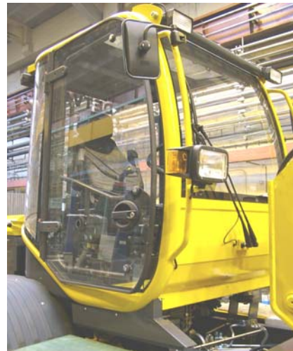
Figure 5. Metal cab final prototype
