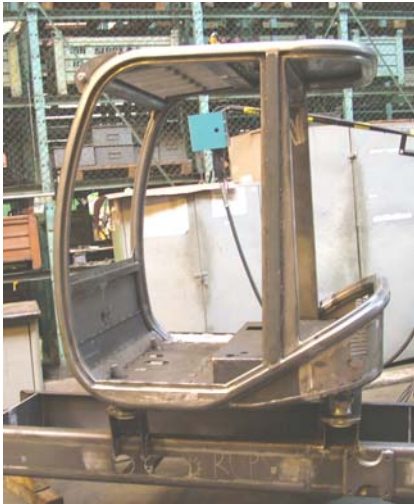
Figure 4. Metal cab body-in-white prototype
