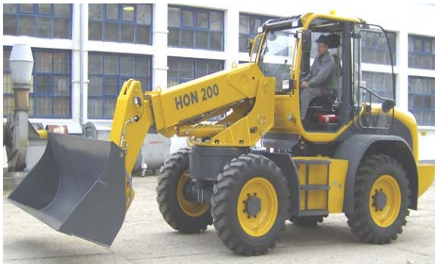
Figure 2. DETVAN HON 200 telescopic manipulator prototype
