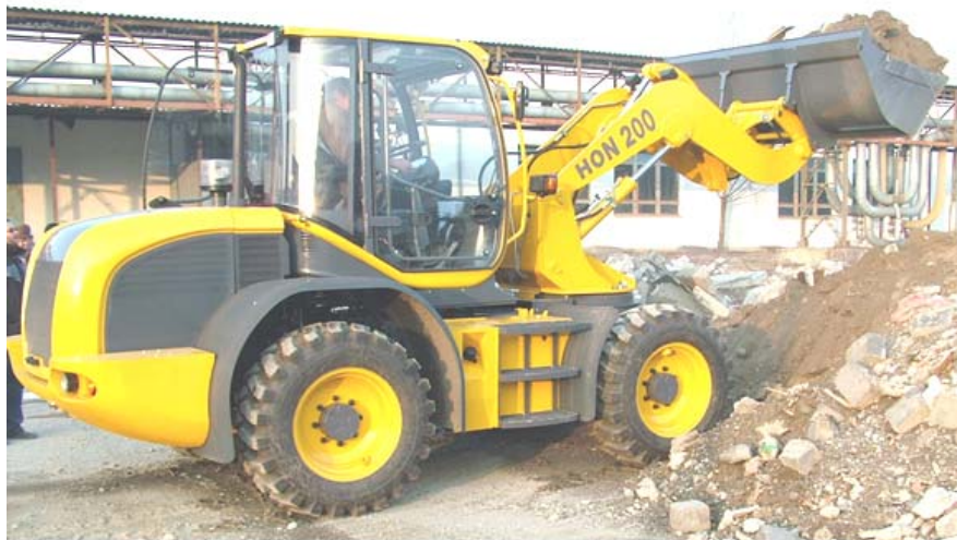
Figure 1. DETVAN HON 200 loader prototype
