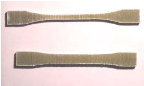
Figure 8: Multi-axial composite specimen
