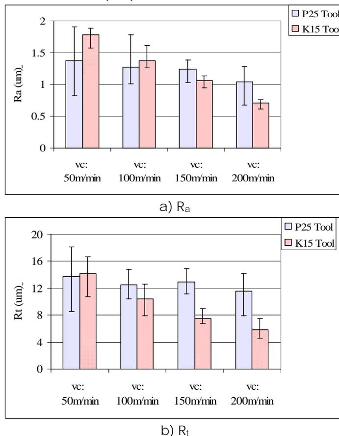
FIGURE 4. Surface roughness when turning of AISI 1045 steel with  $f = 10 \mu m/rev$  and  $a_p = 100 \mu m$  as a function of cutting speed and tool material.
