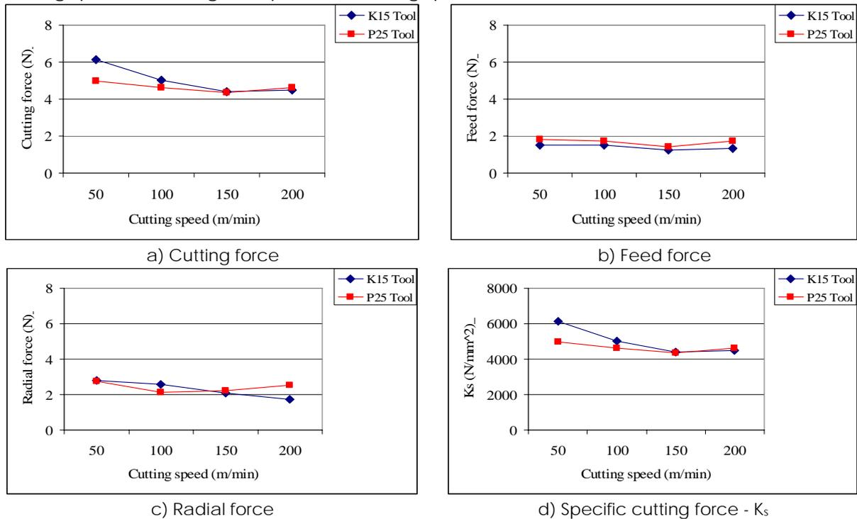
FIGURE 3. Effect of cutting speed on turning forces and specific cutting force when machining of AISI 1045 steel with  $f = 10 \mu m/rev$  and  $a_p = 100 \mu m$  using uncoated (K15) and coated (P25) cemented carbide tools.
