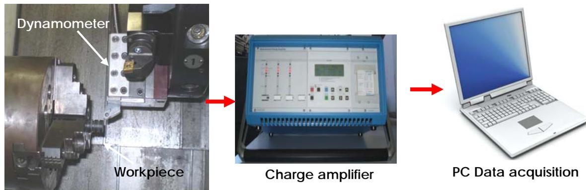
FIGURE 1. Set up for measuring three component turning forces
