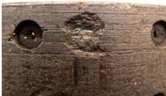
FIGURE 6. Fragment of the frictional lining with a visible abruption on the surface
