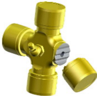
FIGURE 5. Cardanic cross made up by one element
