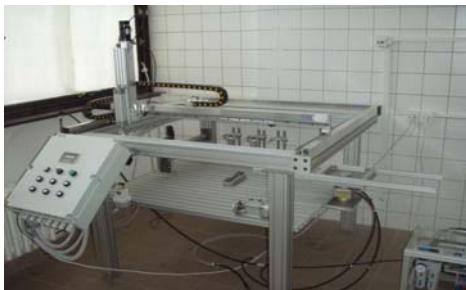
FIG. 2 MODEL OF CARTESIAN ROBOT AND FEEDING DEVICE
