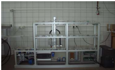
FIG. 3 ASSEMBLED SHELF - STORAGE WITH MANIPULATOR
