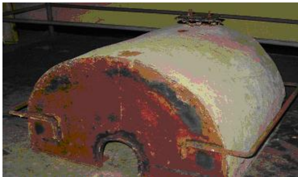
FIGURE 7. The design of the furnace used for warming up the samples
