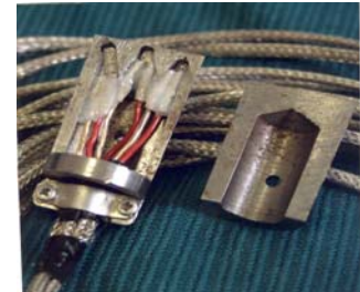
FIGURE 5. The ensemble of thermo – couple bolt in the mounting phase
