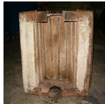
FIGURE 8. The setting of loops inside the electrical furnace
