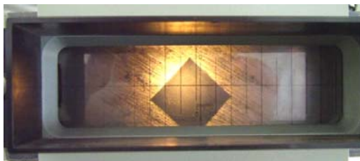
FIGURE 5. A LOOK INTO LENS OF HPO 250 VICKERS HARDNESS TESTER
