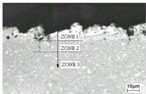
FIGURE 3. HEAT AFFECTED ZONE OF THE SAMPLE AFTER WEDM CUTTING
