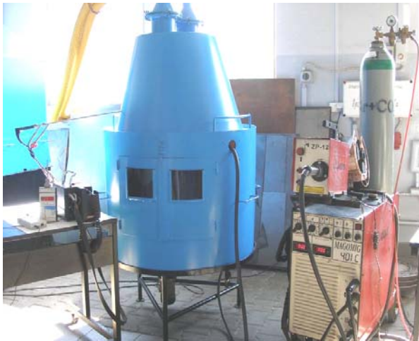
FIGURE 2. Laboratory stand for sampling of dust during MIG/MAG welding of steel
