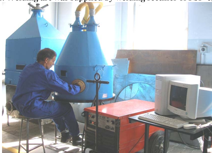
FIGURE 4. Experimental stand for drawing samples of dust generated during MMA welding with covered electrodes
