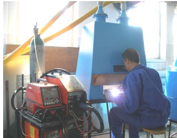
FIGURE 3. Experimental stand for samples drawing of dust emitted while TIG welding of steel
