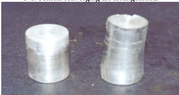
F-3. Extruded Al preform (length of preform=2.63cm; die angle= 6^\circ , reduction ratio=1.6)
