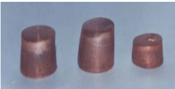
F-4. Extruded copper preform (semi cone angle of the die= 6^\circ , reduction ratio=1.6)
