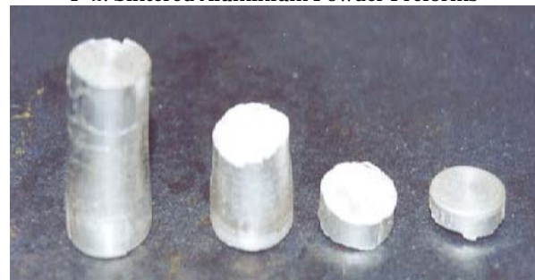
F-3. Extruded Al preform (length of preform=2.63cm; die angle= 6^\circ , reduction ratio=1.6)
