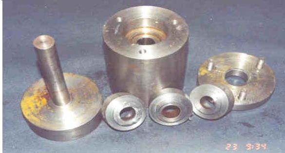
F-1. Conical converging die arrangements
