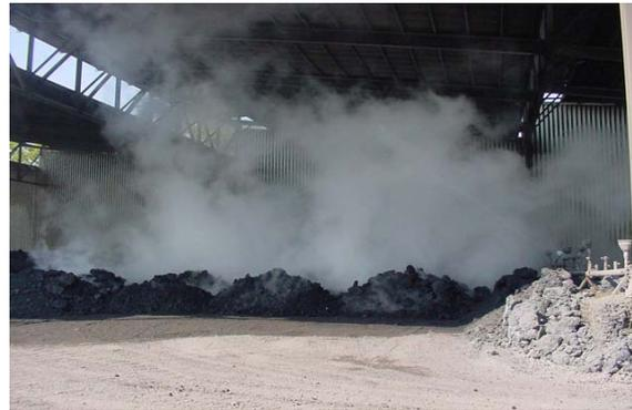
Figure 4. Cooling area with water spraying
