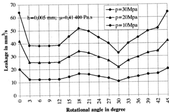
FIGURE 4. Leakage trough a sector in dependent of rotational angle
