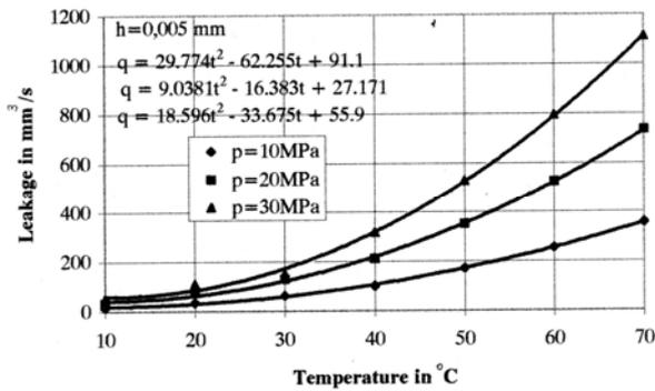
FIGURE 6. Dependence of the valve's plate leakage on the gap
