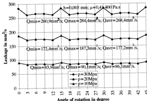
FIGURE 5. Leakage trough valve plate
