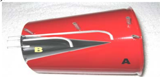
Figure 8. The external axial collector with the internal cone (longitudinal view)
