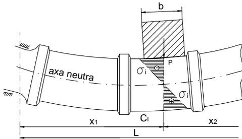
Figure 2. Roll stress caused by rotational bending stress
