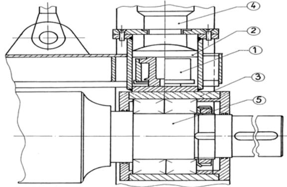
Figure 5. The tensiometer's montage with resistive transducers
