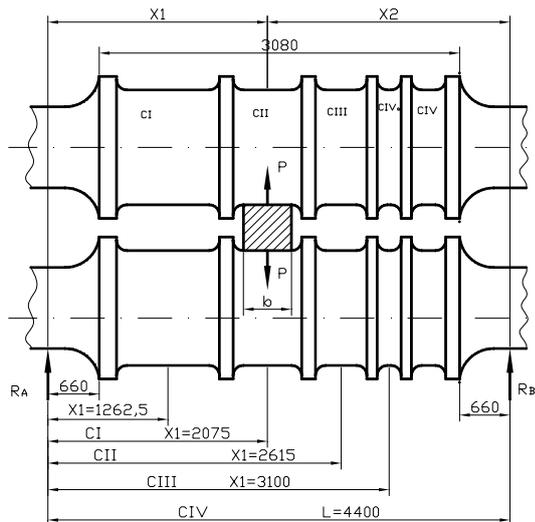
Figure 3. Calculus scheme for the lamination rolls
