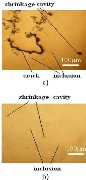
Figure 4. Micrographs of the un-etched samples: a) Piece A and b) Piece D
