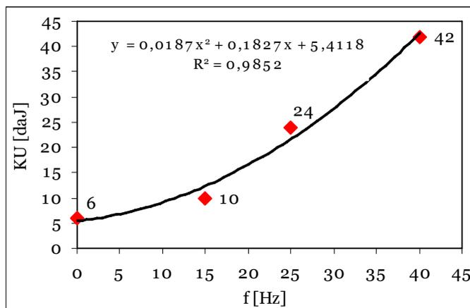
Figure 6. Variation of the energy absorbed trough tearing (KU) with the die vibration frequency (f)
