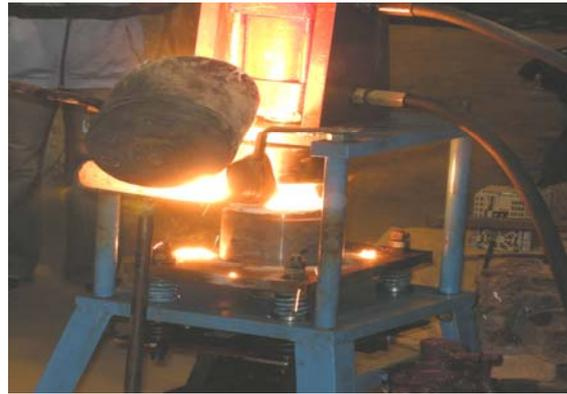
Figure2. Casting of the melt in the die
