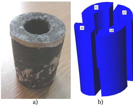
Figure3. Piece A (a) and the cutting way of the samples notated A1-A4 (b)
