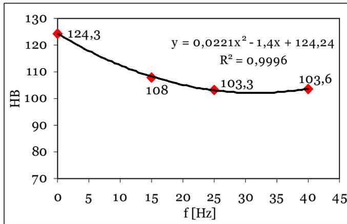
Figure 7. Brinell hardness variation (HB) with the vibration frequency (f) of the die
