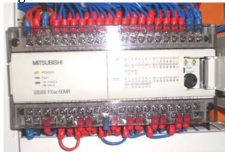
Figure 6. PLC of device for checking plain bearings
