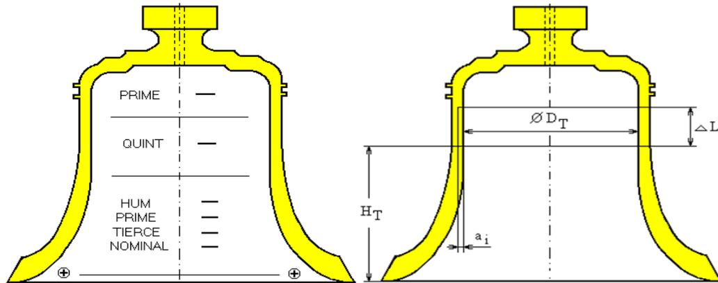
Figure 1. A sketch showing principles of tuning the bells to different tone (a), and the tuning parts of the larger bell (b). Adopted from source [6].
