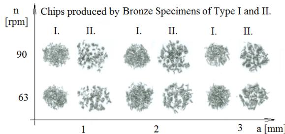
Figure 6. Comparison of chips produced by the Type I and II bronze specimens [6]
