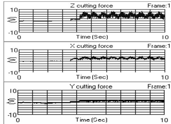
Figure 4. An example of experimental plot for  $F_z$ ,  $F_y$  and  $F_x$  cutting force components obtained from bronze sample (II.), machined at a constant cutting speed of 90 rpm, feed rate of 0.34mm/rev, and depth of cut of 1mm by using a TiN+Ti(C, N) coated carbide insert - Type TNMG 160408QM 215 impounded in a Type 2525M16M1 holder. The overhang of the tool holder was 2 cm. The scale of measurement (0-10 V) is equal to 0-1000 N for  $F_z$ ,  $F_y$  and  $F_x$ .
