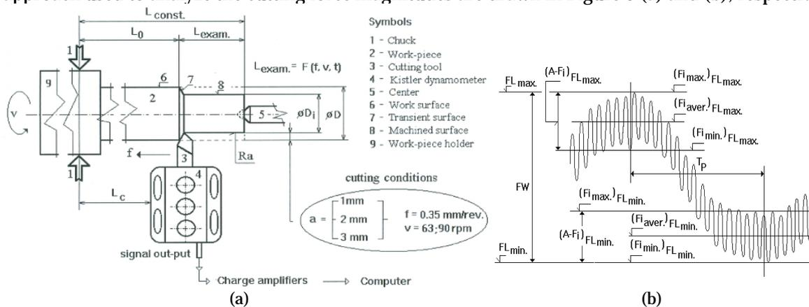
Figure 3. Key elements (forces and amplitudes) to frequency analysis of the dynamic characteristics obtained while machining tin bronzes – bell material [6, 10, 14]. Where the symbol FW represents the width of a frequency signal;  $F_i$  correspond to  $F_x, F_y$  and  $F_z$  cutting force components;  $F_{i\max}$  and  $F_{i\min}$ . Associate with the maximum values of cutting force components ( $F_i - x, y$  and  $z$ ) measured in the minimum level of the frequency chart.
