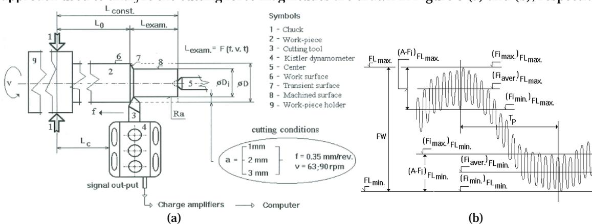
Figure 3. Key elements (forces and amplitudes) to frequency analysis of the dynamic characteristics obtained while machining tin bronzes – bell material [6, 10, 14]. Where the symbol FW represents the width of a frequency signal;  $F_i$  correspond to  $F_x, F_y$  and  $F_z$  cutting force components;  $F_{i\text{max}}$  and  $F_{i\text{min}}$ . Associate with the maximum values of cutting force components ( $F_i - x, y$  and  $z$ ) measured in the minimum level of the frequency chart.
