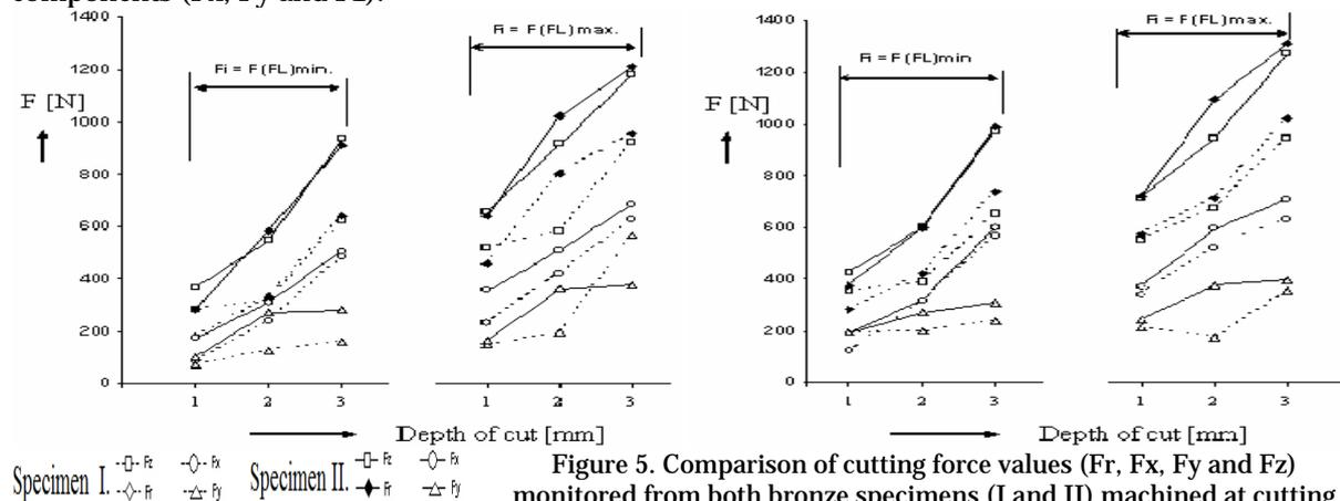
Figure 5. Comparison of cutting force values ( $F_r$ ,  $F_x$ ,  $F_y$  and  $F_z$ ) monitored from both bronze specimens (I and II) machined at cutting speeds of 63 rpm (a) and 90 rpm (b), a feed rate of 0.35 mm/rev, and depths of cut of 1, 2 and 3 mm.
