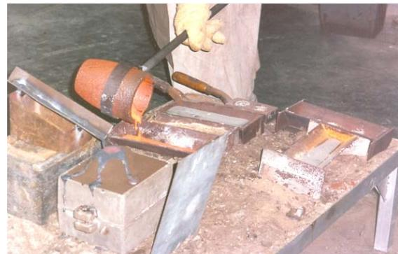
Figure 2. A photograph showing casting different type Cu-Sn specimens in a bar form for metal machining tests [6].
