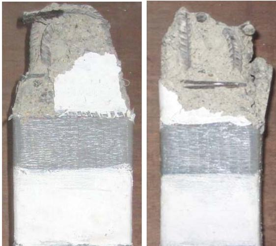
Figure 2(c): Crushing and rupture of FRP strip for repaired specimen CL3
