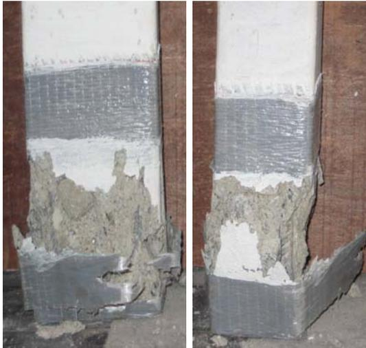
Figure 3(c): Crushing and rupture of FRP strip for repaired specimen CS3
