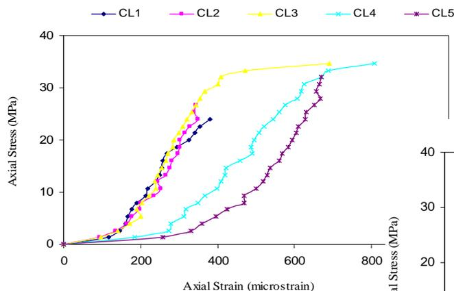
Figure 5: Axial stress-strain curves for control and repaired specimens in series CL
