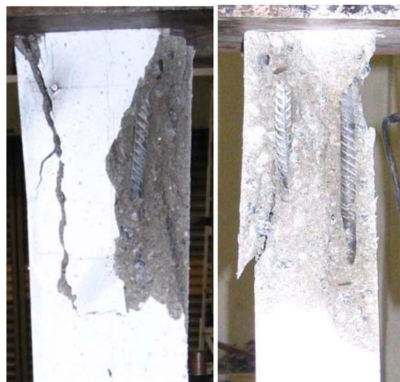
Figure 2(a): Crushing of concrete for control specimen CL1
