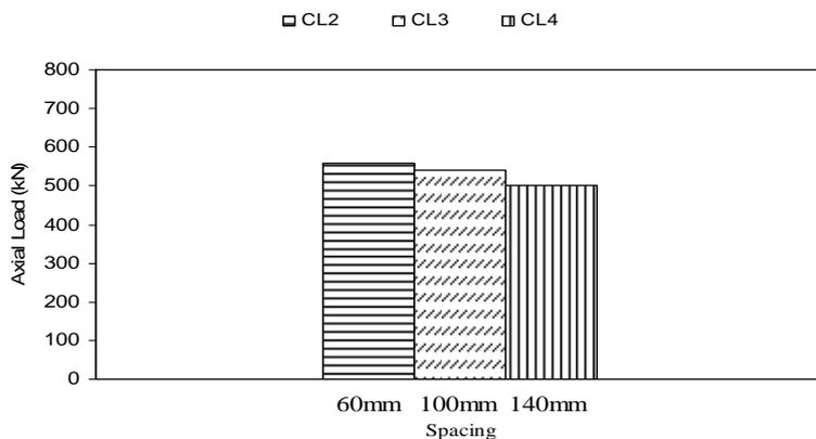
Figure 8: Comparison of compressive load with different spacing (60mm 100mm, and 140mm) of GFRP strips for repaired specimens in series CL
