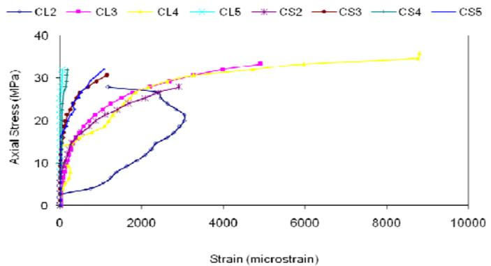
Figure 7: Axial load versus strain in fibres for repaired specimens
