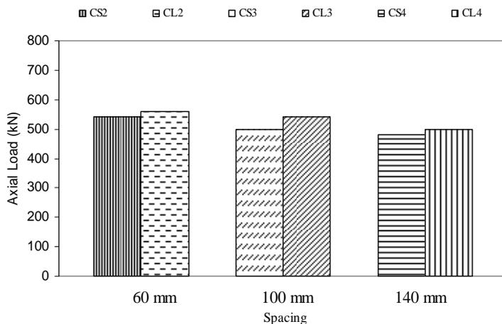
Figure 12: Comparison of compressive load with different slenderness ratio (6.0 and 3.33) for series CL and CS
