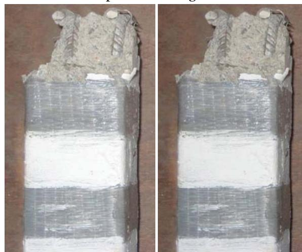
Figure 2(b): Crushing and rupture of GFRP strip for repaired specimen CL2
