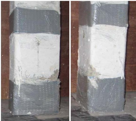
Figure 2(e): Compression failure for repaired specimen CL5
