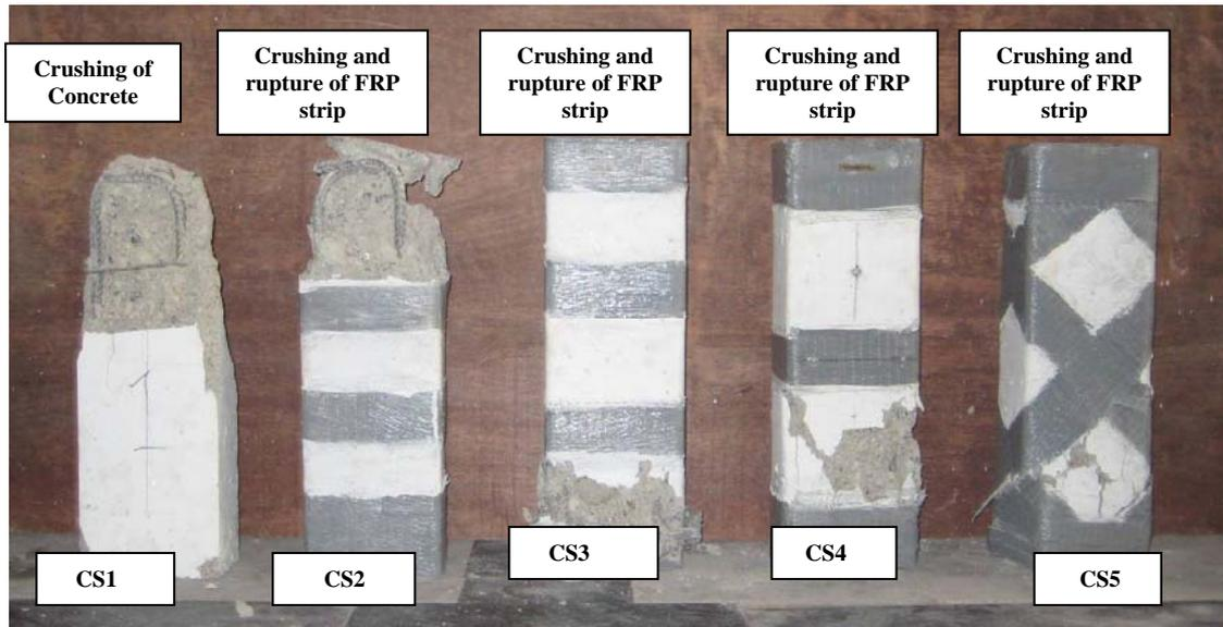
Figure 4(b): Failure patterns for control and repaired specimens in series CS
