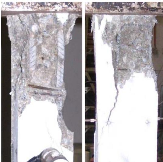
Figure 3(a): Crushing of concrete for control specimen CS1
