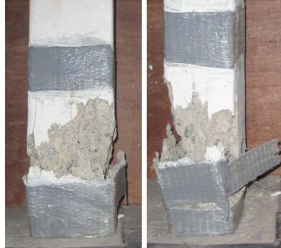
Figure 2(d): Crushing and rupture of FRP strip for repaired specimen CL4
