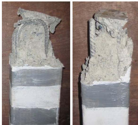
Figure 3(b): Crushing and rupture of FRP strip for repaired specimen CS2
