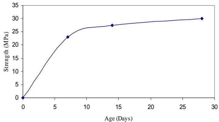
Figure 1. Concrete strength versus time
