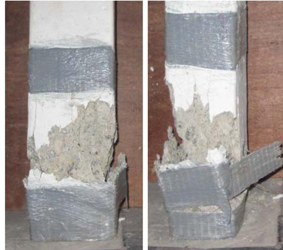
Figure 2(d): Crushing and rupture of FRP strip for repaired specimen CL4
