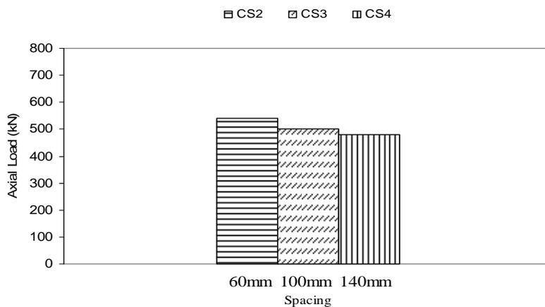
Figure 9: Comparison of compressive load with different spacing (60mm 100mm, and 140mm) of GFRP strips for repaired specimens in series CS
