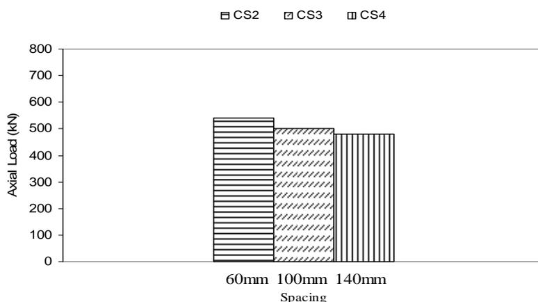
Figure 9: Comparison of compressive load with different spacing (60mm, 100mm, and 140mm) of GFRP strips for repaired specimens in series CS
