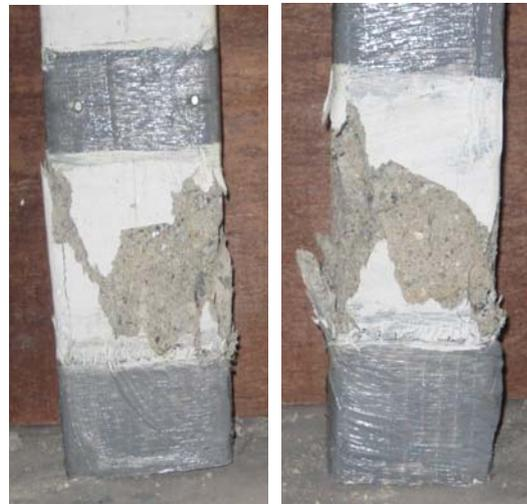
Figure 3(d): Crushing and rupture of FRP strip for repaired specimen CS4
