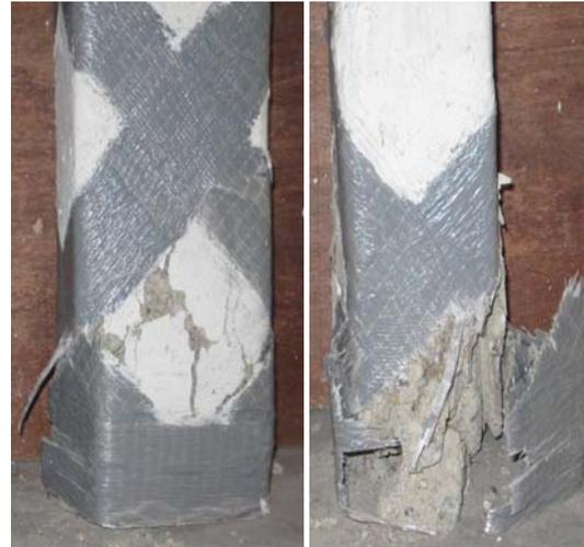
Figure 3(e): Crushing and rupture of FRP strip for repaired specimen CS5
