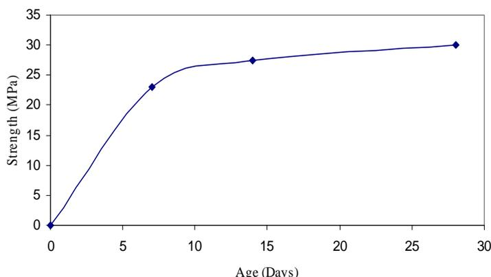
Figure 1. Concrete strength versus time
