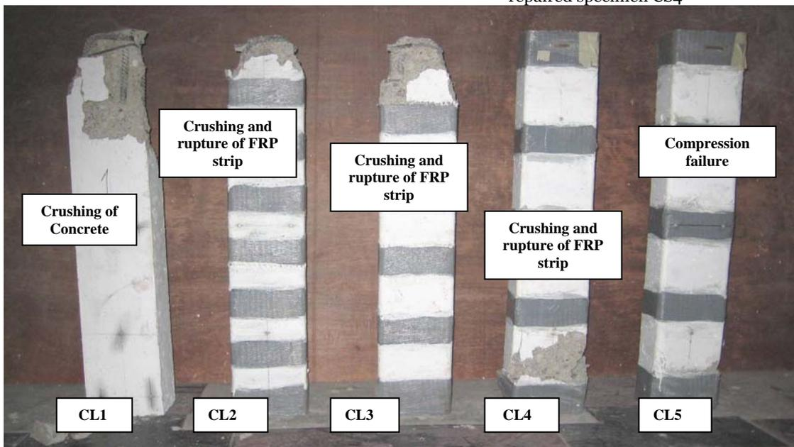
Figure 4(a): Failure patterns for control and repaired specimens in series CL
