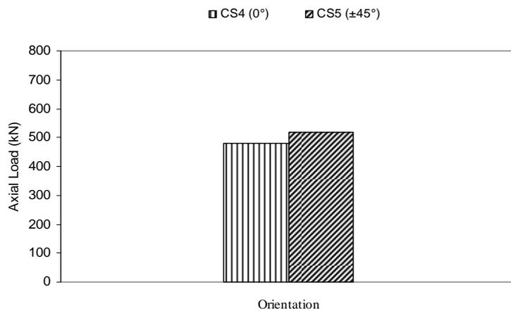
Figure 11: Comparison of compressive load with different fibre orientations (0° and ±45°)
