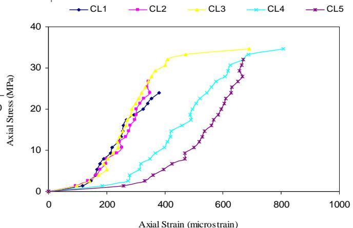
Figure 6: Axial stress-strain curves for control and repaired specimens in series CS
