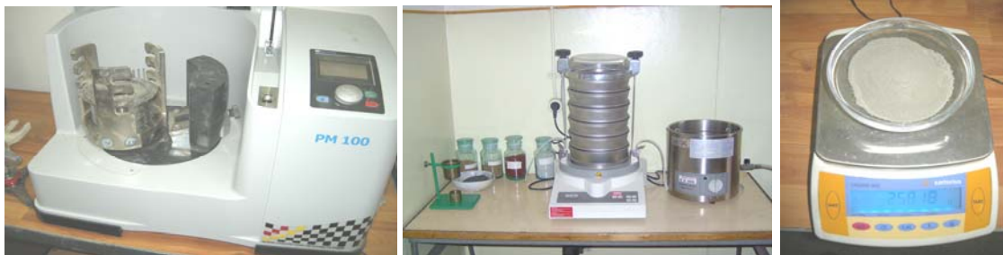
Figure 8. The installations used for clinker production
