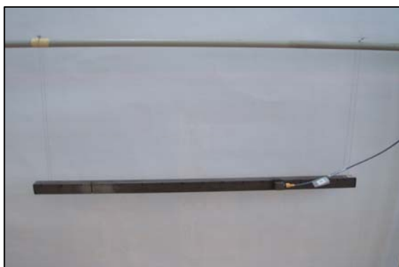
Figure 2. Two boundary conditions: the freely supported beam and the cantilever beam
