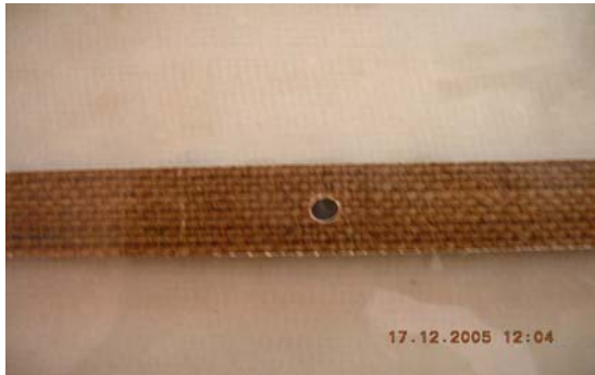
Figure 2. Notched composite specimen
