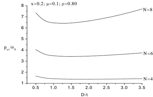
FIGURE (8) VARIATION OF RELATIVE AVERAGE PRESSURE WITH D/t FOR DIFFERENT NO. OF SIDES IN A POLYGON
