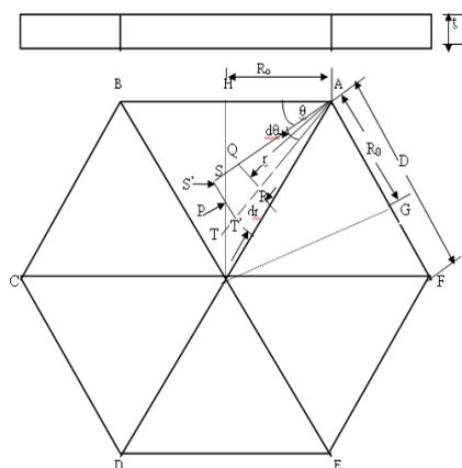
Figure 2. The hexagonal shaped disc with thickness  $t$  and side  $2R_0$
