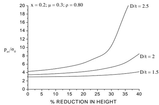
FIGURE (6) INFLUENCE OF D/t RATIO ON RELATIVE AVERAGE PRESSURE ON THE PUNCH WITH PERCENTAGE REDUCTION IN PREFORM HEIGHT
