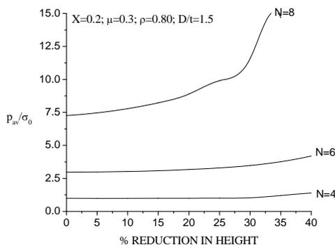
FIGURE (9) VARIATION OF RELATIVE AVERAGE PRESSURE WITH PERCENTAGE REDUCTION IN PREFORM HEIGHT FOR DIFFERENT NO. OF SIDES IN A POLYGON
