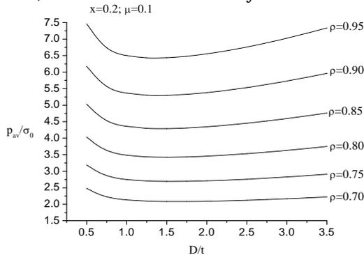
FIGURE (3) VARIATION OF RELATIVE AVERAGE PRESSURE WITH D/t FOR DIFFERENT INITIAL RELATIVE DENSITY OF PREFORM
