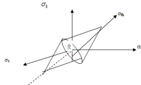
Figure (1) Yield surface for porous metal powder preform
