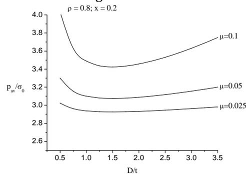
FIGURE (4) EFFECT OF THE CONDITION OF LUBRICATION ON THE RELATIVE AVERAGE PRESSURE FOR VARIOUS GEOMETRIES OF THE HEXAGONAL DISC
