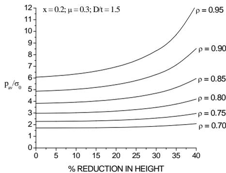
FIGURE (5) VARIATION OF RELATIVE AVERAGE PRESSURE WITH PERCENTAGE REDUCTION IN HEIGHT OF THE HEXAGONAL DISC AT DIFFERENT VALUE OF INITIAL RELATIVE DENSITY
