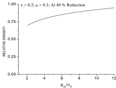
FIGURE (7) VARIATION OF RELATIVE DENSITY WITH RELATIVE AVERAGE PRESSURE ON PUNCH (HEXAGONAL PREFORM)
