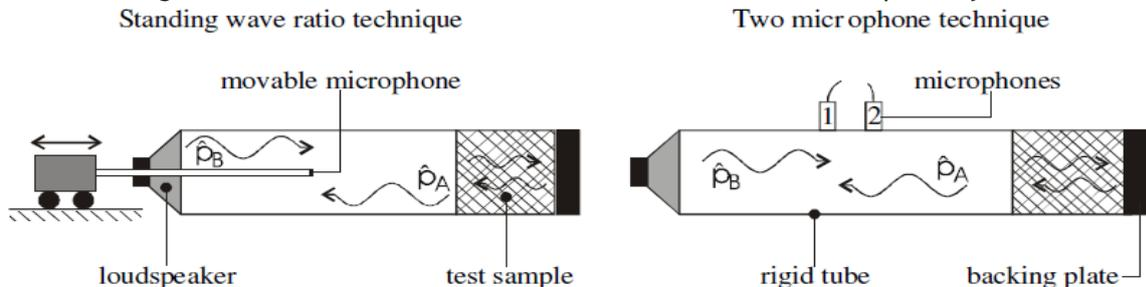
Figure 2 Schematic representations of two measurement techniques in an impedance tube [1]
