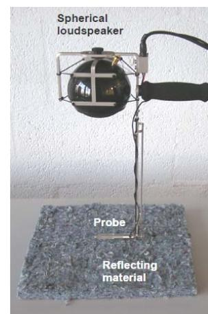
Figure 5 In - situ absorption set up [9]
