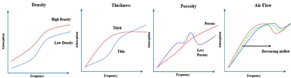
Figure 1 Schematics of the key features driving absorption performance [7]
