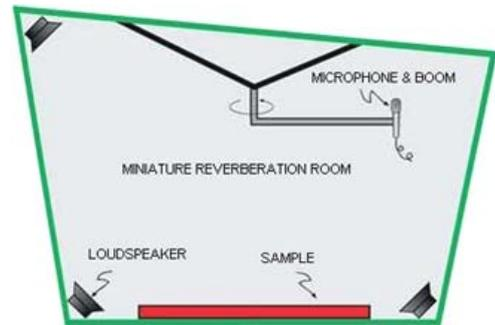
Figure 3 Alpha cabin testing [11]
