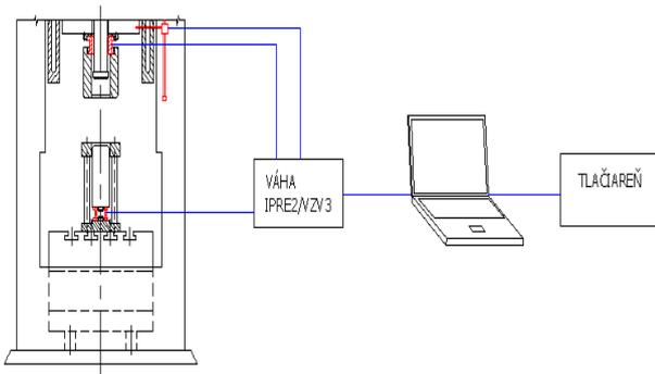
Fig. 1 Scheme of experimental measuring system. Cup, experimental material and experimental forming die
