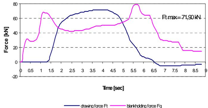
Fig. 5 Course of drawing and blankholding forces,  $D_0 = 134 \text{ mm}$ ,  $m = 0,567$
