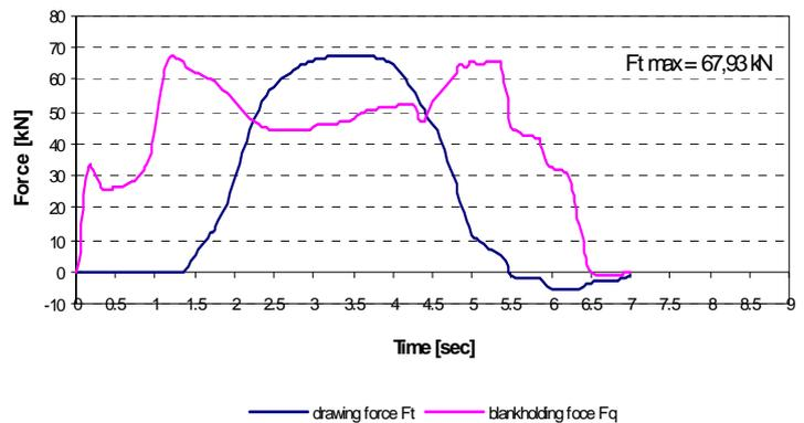
Fig. 4 Course of drawing and blankholding forces,  $D_0 = 125 \text{ mm}$ ,  $m = 0,608$
