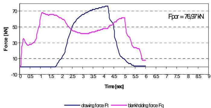
Fig. 7 Course of drawing and blankholding forces at cup breaking  $D_0 = 145 \text{ mm}$ ,  $m = 0,524$
