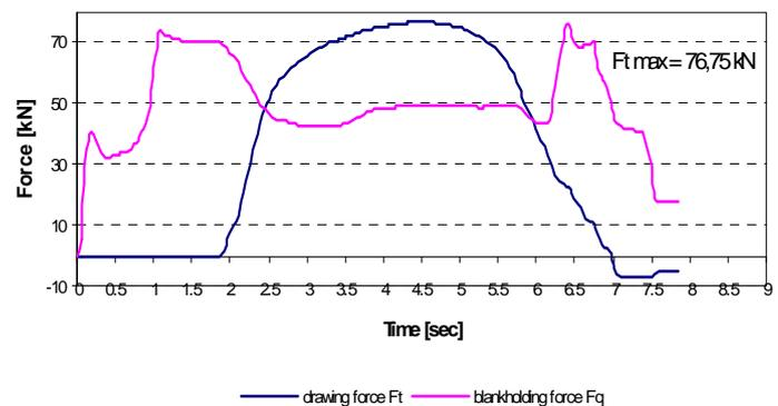
Fig. 6 Course of drawing and blankholding forces,  $D_0 = 139 \text{ mm}$ ,  $m = 0,547$
