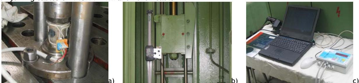
Fig. 3 Components of measuring subsystem for recording forming forces. a) - drawing force dynamometer, b) path reader Mitutoyo SD-60, c) tensometric apparatus IPRE2/VZV3 interconnected with PC
