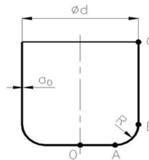
Fig. 2 Experimental flat bottomed cylindrical cup
