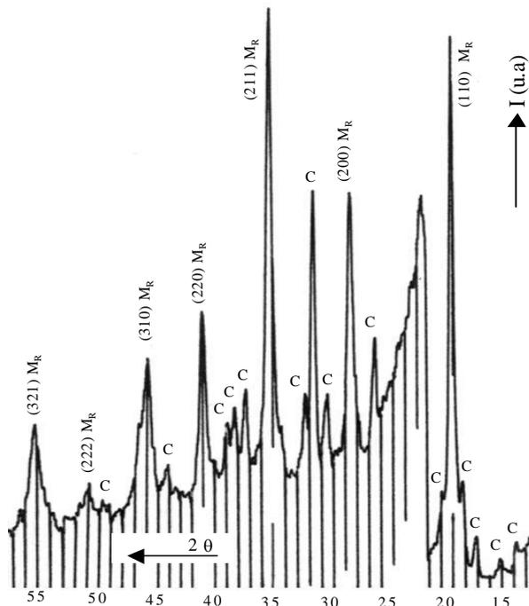
Figure 7: The diffractogram of the status, after tempering3 ( $M_R$  tempering martensite, C -  $Fe_3W_3C$  carbides)
