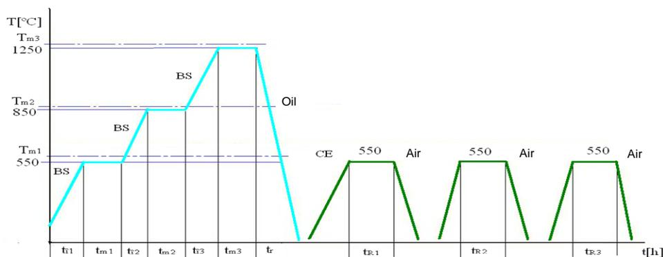
Figure 1. The cyclogram of the secondary heat treatment applied on the HS 18-0-1 steel
