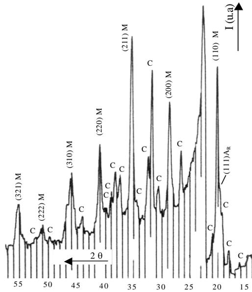
Figure 5: The diffractogram of the quenched status (M-quenching martensite,  $A_R$ - residue austenite, C- $Fe_3W_3C$  carbides)
