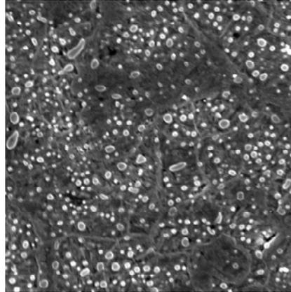
Figure 6. HS 18-0-1 quenched and tempered at 550 °C (x4000)
