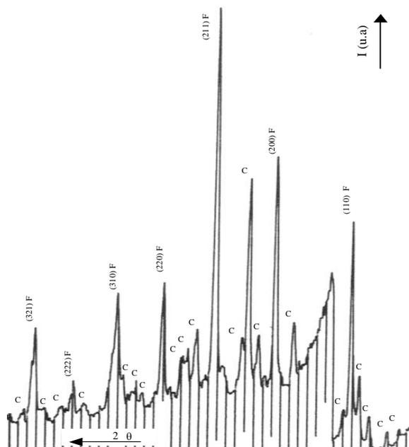
Figure 3: The diffractogram of the annealed status. (F-ferrite, C -  $Fe_3W_3C$  carbides)
