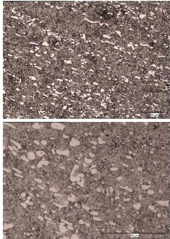
Figure 2. HS 18 - 0 - 1 steel - forged + annealed (Sorbite and, primary and secondary carbides)
