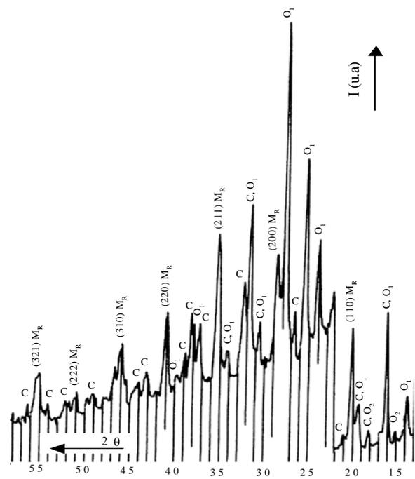
Figure 8: The diffractogram of the ferroxated state ( $M_R$  tempering martensite, C -  $Fe_3W_3C$  carbides,  $O_1$ -  $Fe_3O_4$  oxide,  $O_2$ -  $Fe_2O_3$  oxide)
