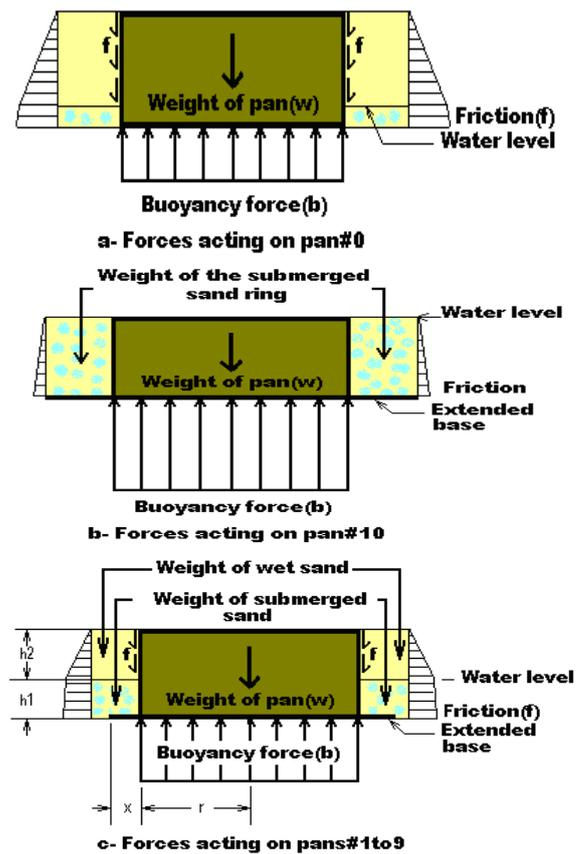
Fig.2 Forces distribution on testing pans
