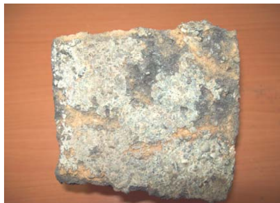
Fig.2. Interface between slag layer and brick
