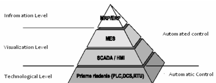
Fig.2. The Layers in the Distributed control system
