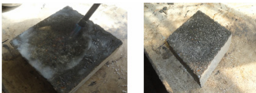
Fig. 3. Water-proofing of concrete by Wax
