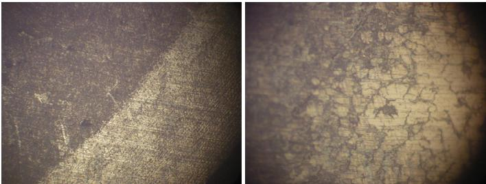
Hardened layer depth, is about 4 mm for specimens of steel and approximately 3.5 mm for specimens of steel. Are normal differences between hardened layer depth and hardness differences because steel 41Cr4 steel has a greater hardenability as 34CrMo4 steel (higher carbon content and boron contains increases hardenability).
