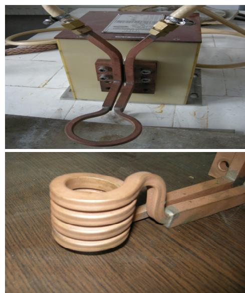
Fig.6. Tempering transformer and inductor
