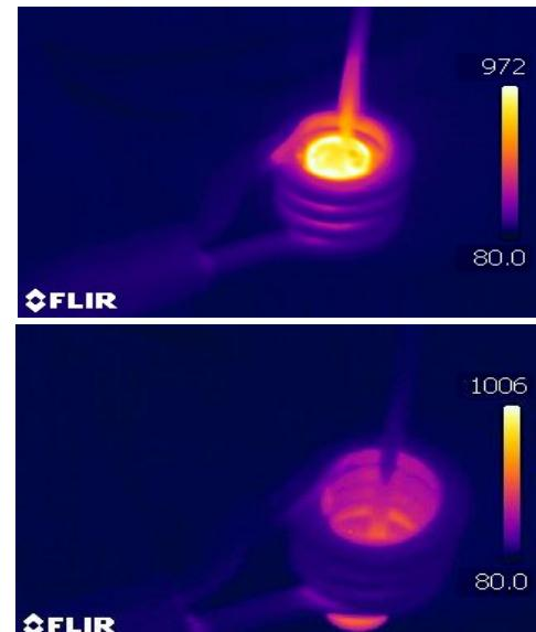
Fig. 7. Temperature of pieces measured with thermographic cameras
