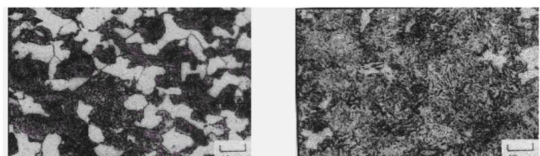
Fig.3. Steel microstructure 1C45 (AISI 1045) before and after the induction surface hardening
