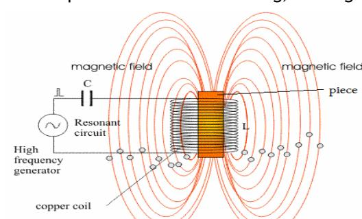
Fig.5 Work principle for induction heating
