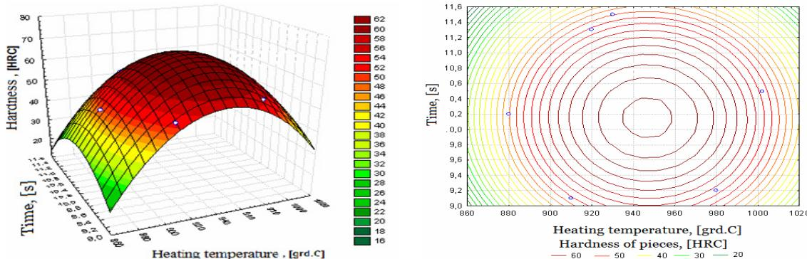
Fig. 11. Hardness variation for pieces made from 34CrMo4 steel, cumulative value
