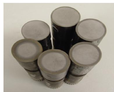
Fig. 2. Some pieces with different hardening depth depending of generator power, frequency and maintained time in inductor
