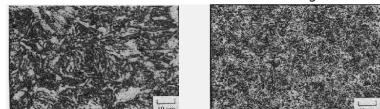
Fig.4. Steel microstrucrure 42CrMo4 (AISI 4140) before and after the induction surface hardening
