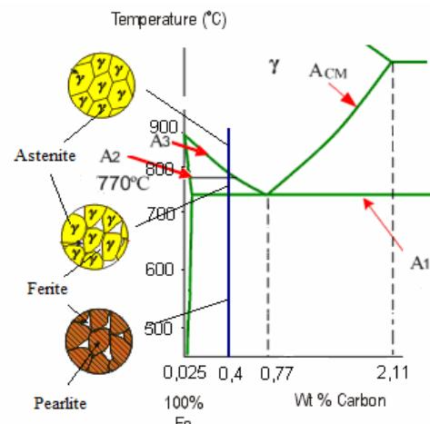
Fig.1. Fe-Fe<sub>3</sub>C diagram, steel area
