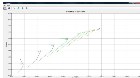
Fig. 11. Fuel Consumption Variation versus Engine Torque and Speed
