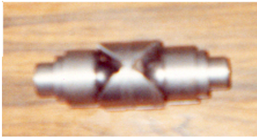
Fig. 6. Active elements of the indexing device
