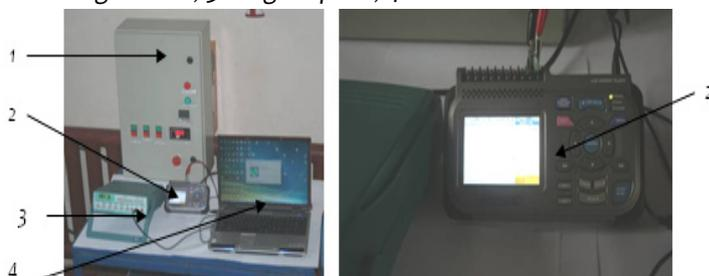
Fig. 7 - Command and control system. 1 – control panel; 2 – data acquisition system with oscilloscope; 3 – signal generator; 4 – laptop data processing
