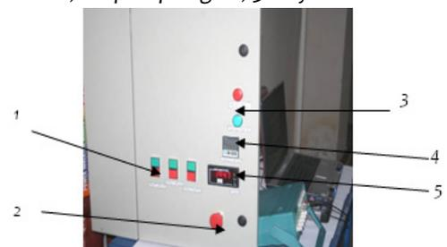
Fig. 8 - Control panel. 1 – on / off buttons; 2 – failure button; 3 – indicator lamps; 4 – oil temperature regulator; 5 – digital display strain gauge signal
