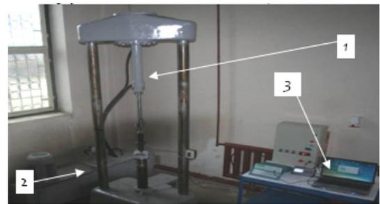
Fig. 4 - Compact Platform for Testing of Dampers (stand). 1 –mechanical system; 2 – hidraulic system; 3 – command and control system
