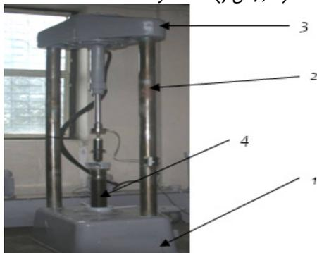
Fig. 5 - Mechanical system. 1 – bed frame; 2 – column guidance; 3 – higher pillar; 4 – driver screw
