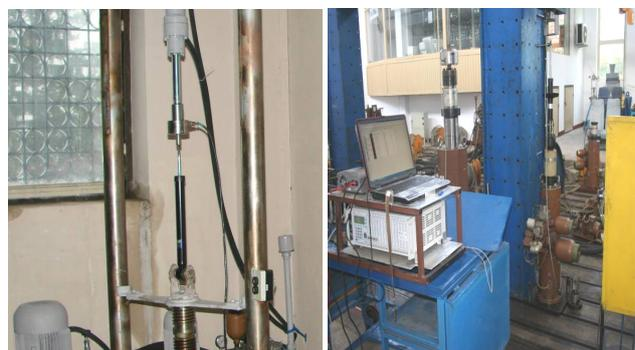
Fig. 10 - Bitubular damper testing for road vehicles - type 1 on Compact Platform for Testing of Dampers - CPTD (left) and on HIDROPULS installation (right)
