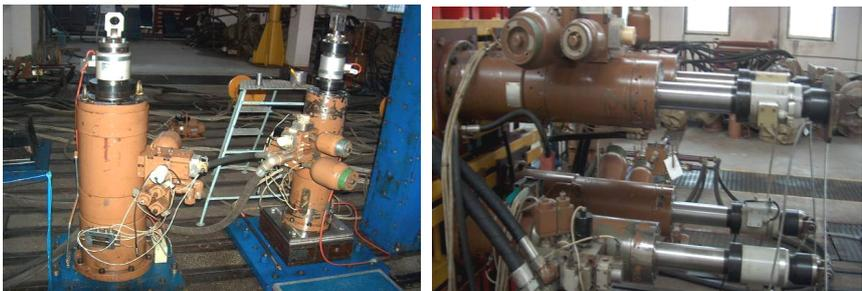
Fig. 2 - Hydraulic cylinders, disposed for operating on vertical and horizontal structures;
