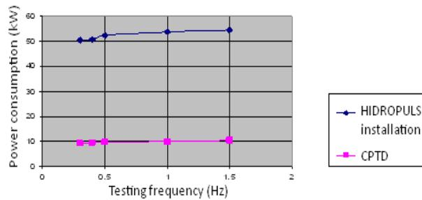
Fig. 12. Comparative consumption for bitubular damper
