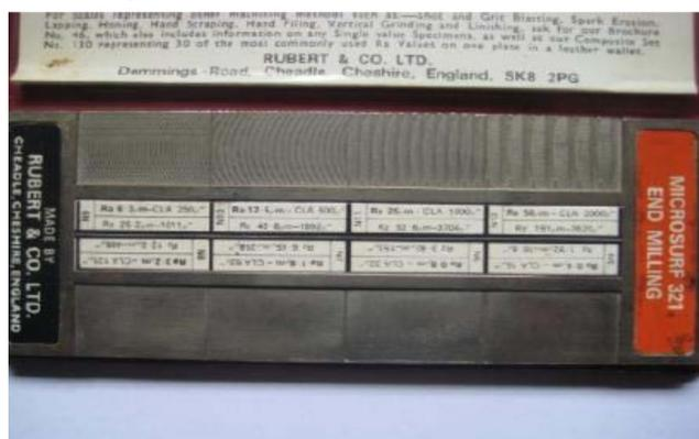
Figure 2. Calibrated end milled plate from Rubert & Co.
