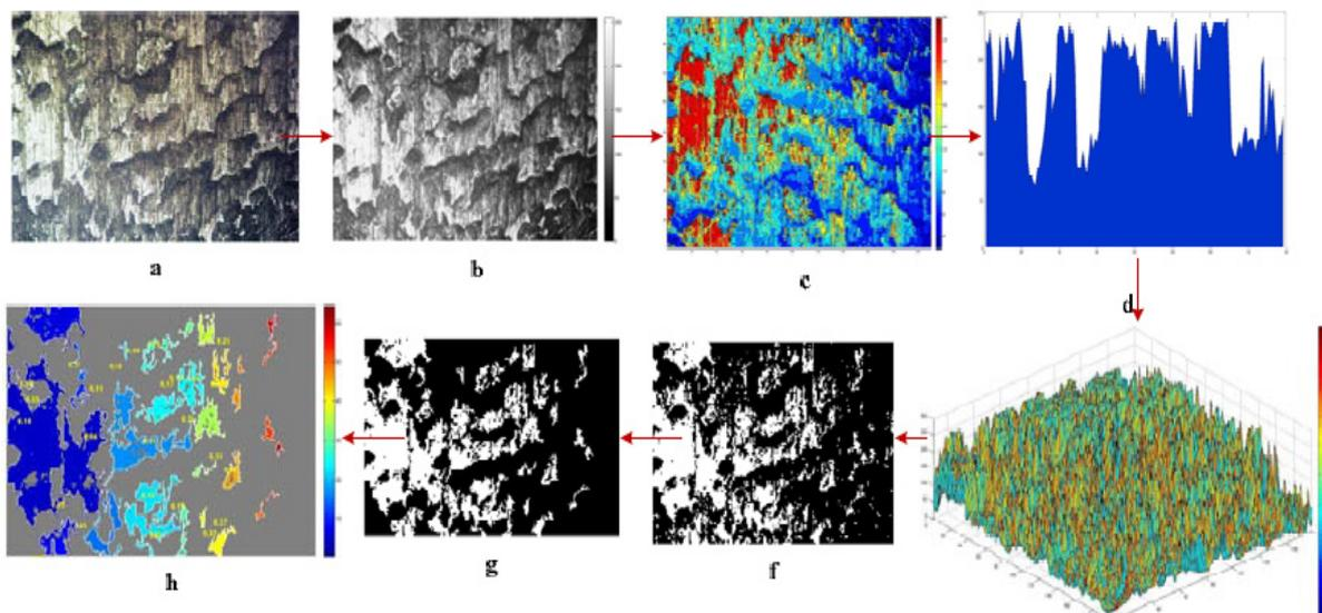
Figure 6. DIP results (horizontal milled plates): (a) 40x zoom RGB micrograph, (b) grayscale, (c) 2-D contour plot, (d) 3-D contour plot, (e) 3-D colored contour plot, (f) black & white image, (g) noise reduction, (h) edge detection
