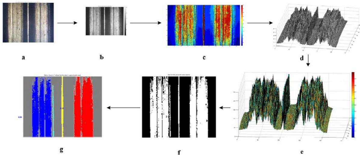
Figure 4. DIP results (shaped plates): (a) 40x zoom RGB micrograph, (b) grayscale, (c) 2-D contour plot, (d) 3-D contour plot, (e) 3-D colored contour plot, (f) black & white image, (g) edge detection
