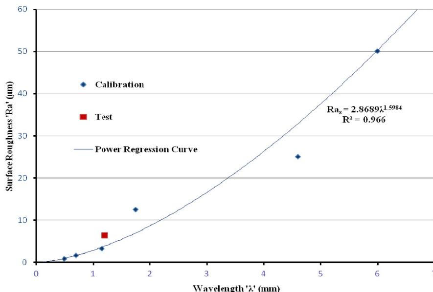
Figure 7. Calibration curve of average surface roughness vs. wavelength of roughness crests for shaped plates
