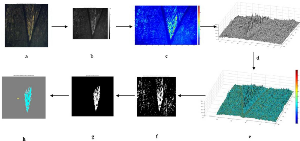
Figure 5. DIP results (end milled plates): (a) 40x zoom RGB micrograph, (b) grayscale, (c) 2-D contour plot, (d) 3-D contour plot, (e) 3-D colored contour plot, (f) black & white image, (g) noise reduction, (h) edge detection
