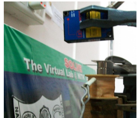
Figure 4. Experiment setup with Laser Pickup (optoNCDT).
