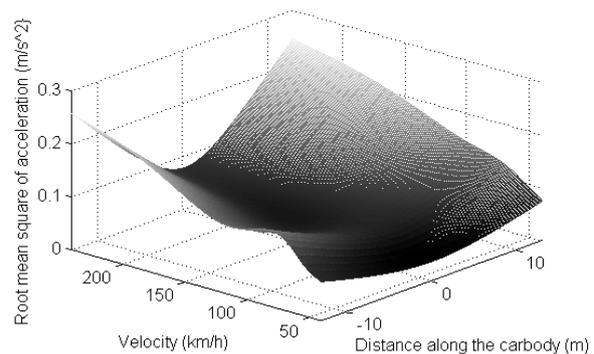
Fig. 8. The RMS value of the car body acceleration ( $\zeta_b = 0.245$ ,  $\zeta_c = 0.180$ ).
