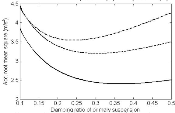
Figure 5. Optimal damping ratio of the primary suspension: —, 120 km/h, ---, 180 km/h, - · - · -, 240 km/h.
