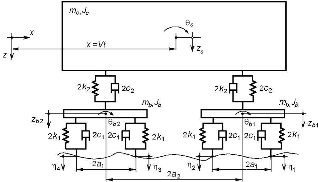
Fig. 1. The vehicle's mechanical model.
