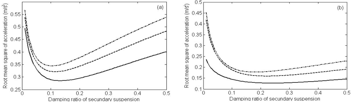
Figure 7. Optimal damping ratio of the secondary suspension (above bogie): a) non-filtering effect; b) filtering effect; —, 120 km/h, ---, 180 km/h, - · - · -, 240 km/h.
