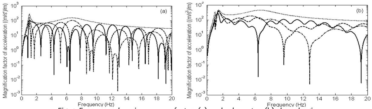
Fig. 4. Frequency-domain response factor: (a) car body center; (b) above bogie
