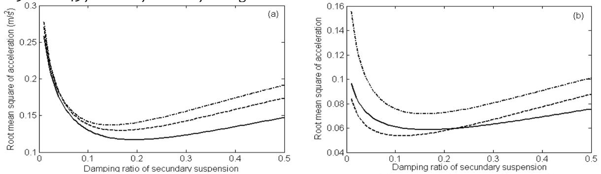
Figure 6. Optimal damping ratio of the secondary suspension (at middle): a) non-filtering effect; b) filtering effect; —, 120 km/h, ---, 180 km/h, - · - · -, 240 km/h.
