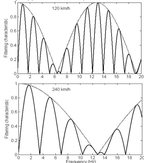
Figure 3. The filtering characteristic above the bogie (the car body pitch).
