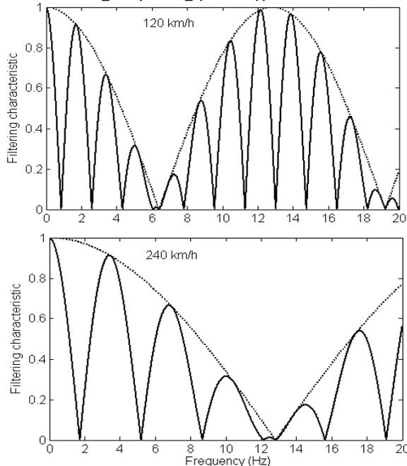
Figure 2. The filtering characteristic in the car body center (bounce).
