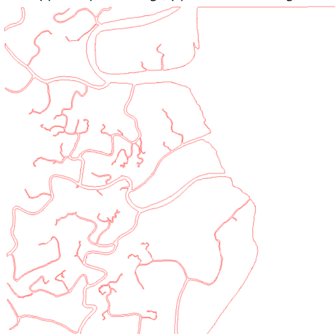
Figure 6. Extracted rivers boundary by snake method
