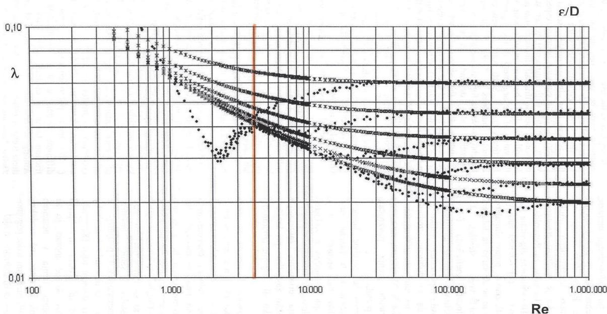
Figure 3. Colebrook-White equation and Nikuradse's measurements [2]
