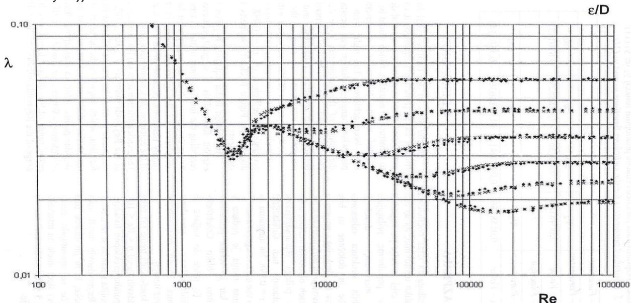
Figure 4. New (generalized) equation for  $\lambda$  and Nikuradse's results [13]
