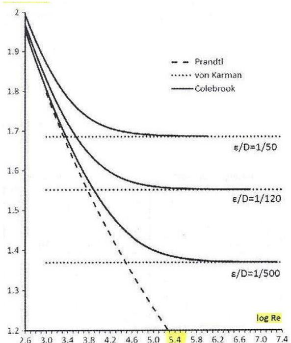
Figure 2. Colebrook-White equation and its components [2]
