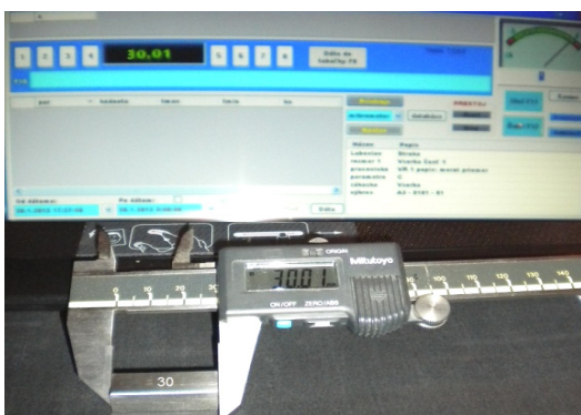
Fig. 1 The verification test of measurement equipment capability index a digital micrometer with using Johansson gauge blocks
