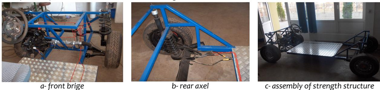
Figure 1. Strength structure of the rolling chassis
