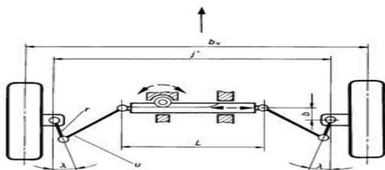
Figure 2. Scheme design of the steering system with pinion-rack mechanism
