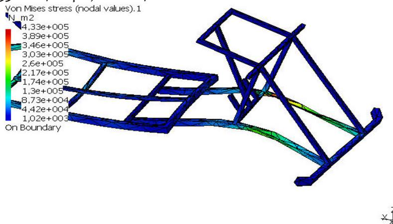
Figure 11. Von Mises equivalent stresses and strength structure deformation after mounting the rolling chassis all stock internal combustion engine and fuel tank
