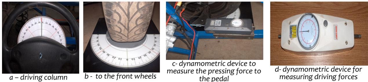
Figure 4. Installation of measuring tools to measure geometric parameters steering the rolling chassis
