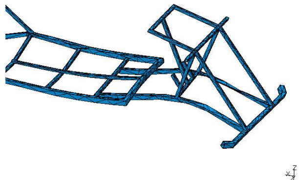
Figure 10. The deformation of the strength structure of rolling chassis
