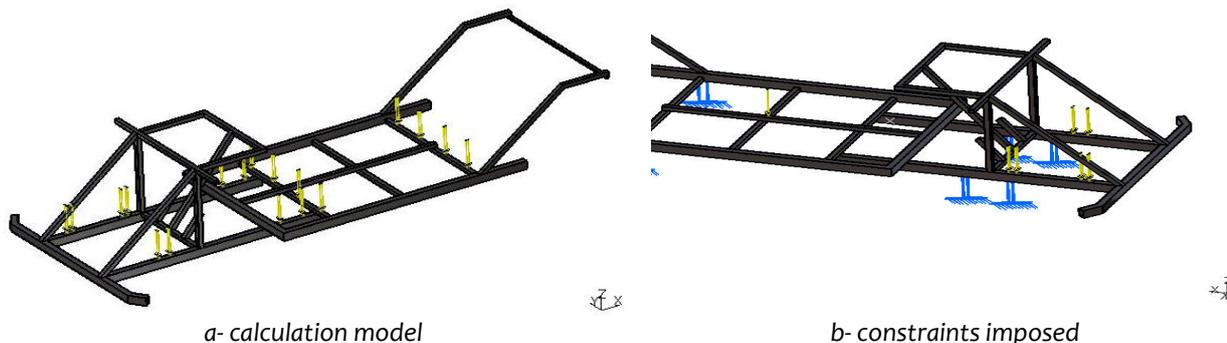
Figure 6. The calculation model of the strength structure of the rolling chassis
