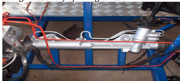
Figure 3. The mounting with pinion – rack mechanism in assembly of the rolling chassis
