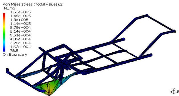
Figure 7. The value of von Mises equivalent stresses and its distribution in the area of strength structure of rolling chassis
