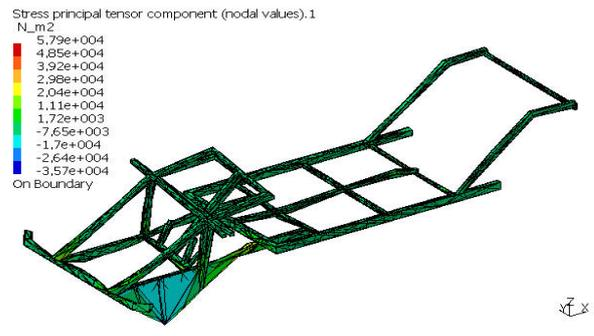
Figure 8. The main value of stresses and its distribution in the area of strength structure of rolling chassis
