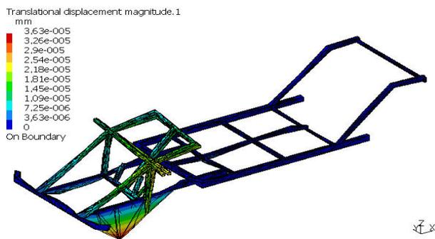
Figure 9. The movements in the whole strength structure of rolling chassis
