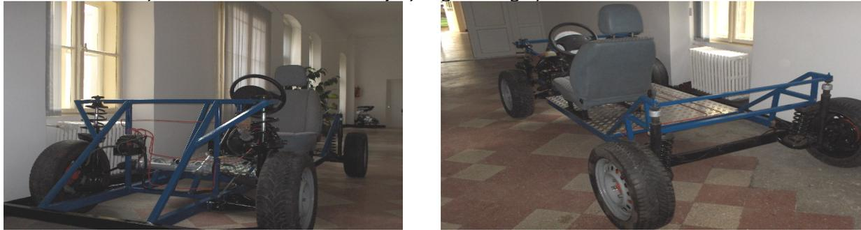
Figure 5. Rolling chassis assembly with mechanical steering system and braking system with aggregate ABS
