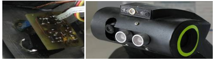
Fig. 5 Infra sensor in robot body, ultrasonic sensor in monitoring head
