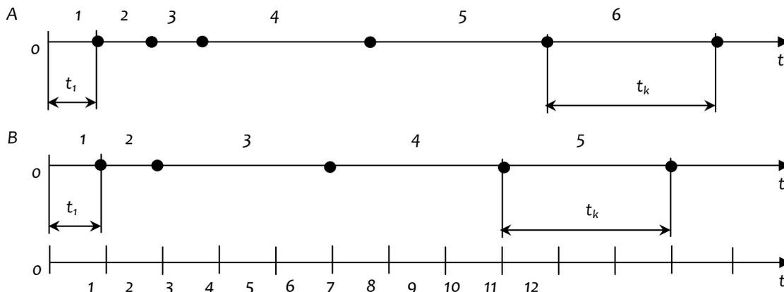
Figure 3: Two different cases of the failure rate development for repaired objects
