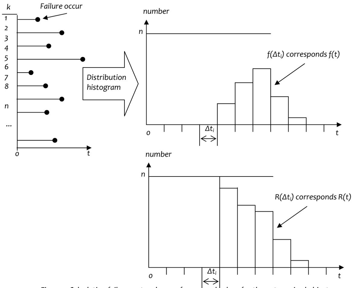
Figure 1: Calculating failures rate scheme of measured values for the not repaired objects.
