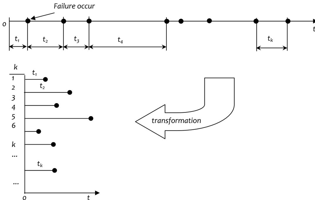
Figure 2: Time record transformation repaired faults into the not repaired type of faults
