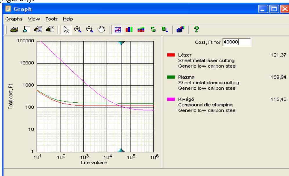
Figure 4. The manufacturing costs vs. life volume.
