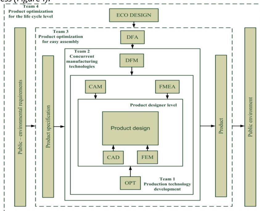
Figure 1. Product design vs. requirements vs. design techniques
