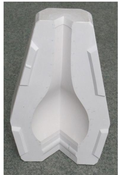
Figure 2. Casting form, made with the prototype core
