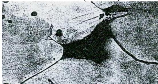
Figure 10. Austenitic structure ( $\times 500$ ). Micro cracks and un-dissolved white carbides ( $P = 0.139\%$ )
