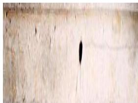
Figure 2. Heat cracks ( $P = 0.134\%$ ), appeared during at the thermal treatment
